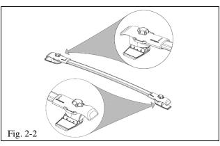
(b) Loosen the clamps by turning the knobs counterclockwise until the lower clamp can be moved from inside of the upper clamp pocket (Fig. 2-2).
